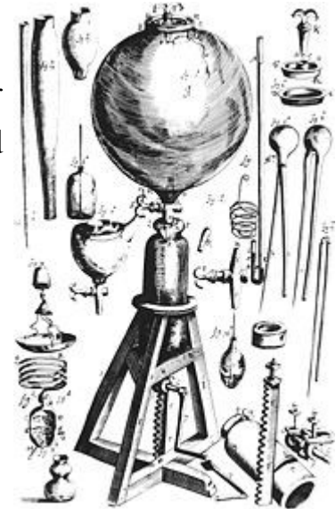
Illustration of an air pump used by Robert Boyle for gas pressure experiments in the 1600s.
