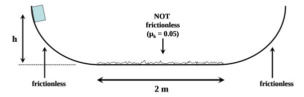
(a) The block is released, makes its first trip to the right hand side, returns to the left hand side, and then returns once more to the right. On this second excursion to the right side, how high up the ramp does the block go?
