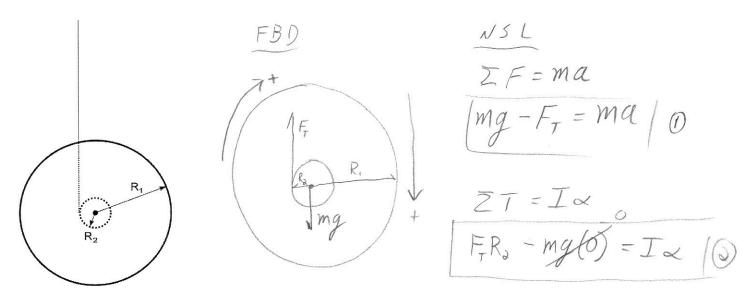
We need the linear acceleration, a, of the yo-yo. Let's eliminate F, From equations () and (), then solve For a:
