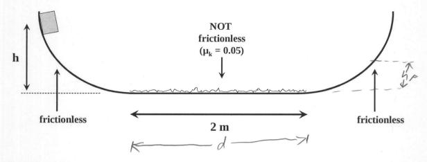
(a) The block is released, makes its first trip to the right hand side, returns to the left hand side, and then returns once more to the right. On this second excursion to the right side, how high up the ramp does the block go?
