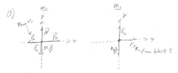
The Frictonal Force From the M. M. interFace is what accelerates block 2, but the presence of block 2 must cause opposition to block 15 acceleration.
