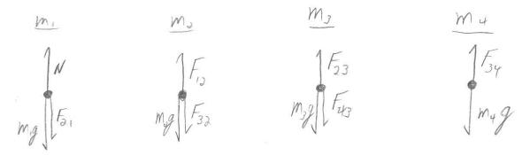
b) Rank the reaction forces from the free body diagrams above in order of magnitude, greatest first. If any are equal, place an equals sign between them.
