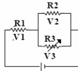
1.4) Type A light bulbs can be wired across a potential difference of up to 100 volts without burning out. Type B bulbs can only be wired across a potential difference of up to 50 volts without burning out. Which of the circuits here would emit the most amount of light without burning out a bulb? (Ignore changes in bulb properties with temperature.)
