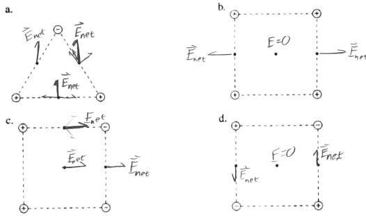
Draw the electric field vector at the three points marked with a dot. Hint:Use symmetry to determine if horizontal or vertical components cancel out.
