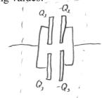
$$C_{eFF} = \frac{Q_{tot}}{\Delta V_{ob}} = \sum \Delta V_{ob} = \frac{Q_{tot}}{C_{eFF}} = \frac{Q_{o} + Q_{o}}{C_{o} + C_{o}} = \frac{645 \text{mC}}{430 \text{mF}} = \boxed{1.5 \text{ V}}$$
