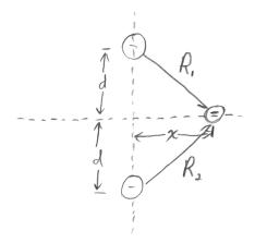
$$U_{net} = \frac{k(-q)(-q)}{R_1} + \frac{k(-q)(-q)}{R_2}, \quad R_1 = R_2 = (\chi^2 + d^2)^{1/2}$$
