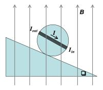
Big hint: Draw a free-body diagram for the sphere. Label gravity acting at the center of mass and calculate its torque relative to the contact point with the incline. Then label the external field and the loop's magnetic moment. The net torque (clockwise vs. counterclockwise) must be zero.
