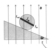
Big hint: Draw a free-body diagram for the sphere. Label gravity acting at the center of mass and calculate its torque relative to the contact point with the incline. Then label the external field and the loop's magnetic moment. The net torque (clockwise vs. counterclockwise) must be zero.
