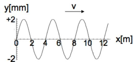
A string is vibrating at 300 Hz. Using a strobe light and an ultra fast camera you get a picture of the string as sketched below. The walls are separated by 1 meter. If the string were vibrating in its lowest possible frequency, what would that frequency be?
